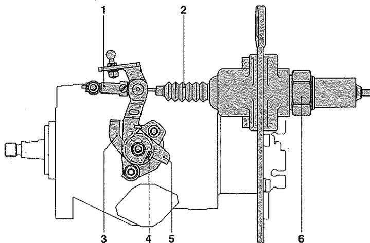
causes the stop lever, the shaft, the inner lever and the ball pin, to swivel and change the roller ring's setting so that the start of delivery is advanced. The ball pin engages in a slot in the roller ring, which means that the timing-device piston cannot rotate the roller ring any further in the "advance" direction until a given engine speed has been exceeded.
