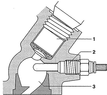
**Fig. 2: Sheathed-element glow plug**
