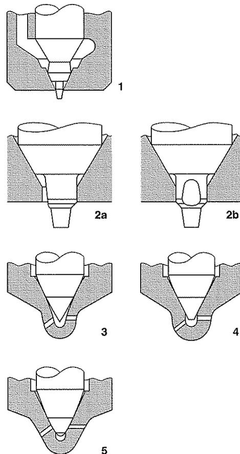
The nozzle cone's mechanical integrity is the limiting factor in the length of the spray hole. At present, spray-hole length is 0.6 ... 0.8 mm in the case of the cylindrical and conical blind holes. With the seat-hole nozzle, the minimum spray-hole length is 1 mm, whereby special hole-making techniques must be applied.
