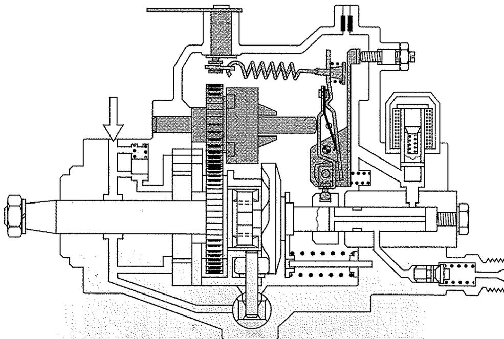
– Maximum-speed governing: With the accelerator pedal fully depressed, the maximum full-load speed must not increase to more than high idle speed (maximum speed) when the load is removed. Here, the governor responds by shifting the control collar back towards the “Stop” position, and the supply of fuel to the engine is reduced.
