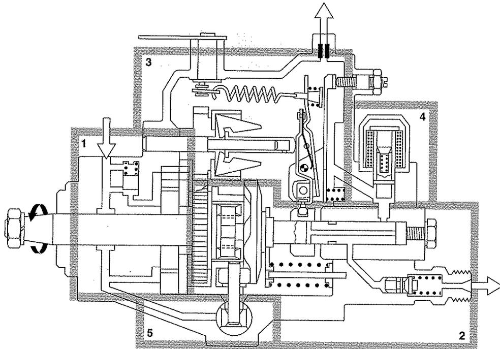
the pump at right angles to the pump's longitudinal axis. Its operation is influenced by the pump's internal pressure which in turn is defined by the vane-type fuel-supply pump and by the pressure-regulating valve. The timing device is closed off by a cover on each side of the pump (Figs. 2 and 3).
