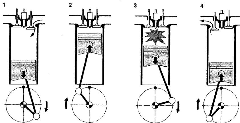
the piston moves up again and drives out the burnt gases through the open exhaust valve.
