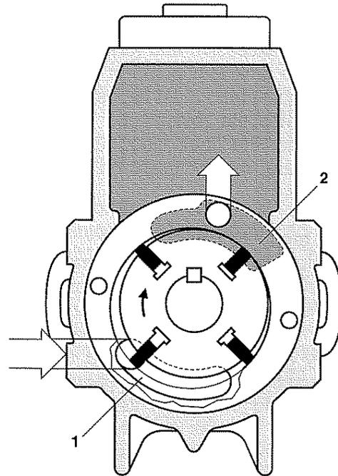
**Fig. 4: Vane-type fuel-supply pump with impeller on the drive shaft.**
