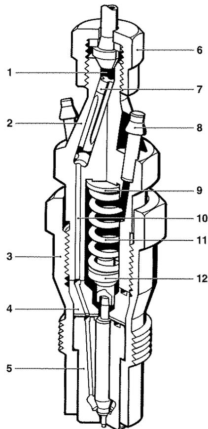
same time sealing against high injection pressures. At the combustion-chamber end, the nozzle needle has a sealing cone which is forced by the pressure spring against the nozzle body's conical sealing surface when the nozzle is closed. The sealing cone's opening angle is slightly different to that of the nozzle body's sealing cone, with the result that linear contact with high compression and good sealing properties is formed between them.
