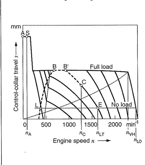
spring attached to the governor housing, this means that idle speed can be adjusted independent of the accelerator-pedal setting, and can be increased or decreased as a function of temperature or load.
