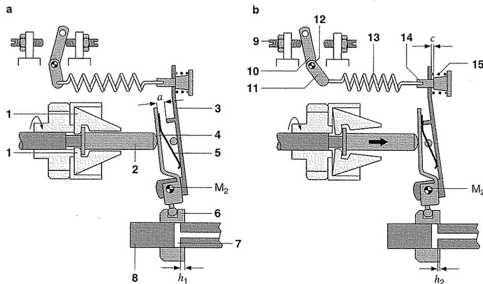
start-quantity position by the ball pin on the starting lever. This means that when the engine is cranked the distributor plunger must travel through a complete working stroke (= maximum delivery quantity) before the cutoff bore is opened and delivery ceases. Thus the start quantity (= maximum delivery quantity) is automatically made available when the engine is cranked.
