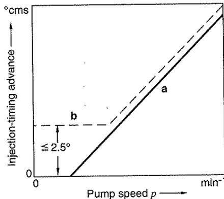
**Fig. 14: Mechanical cold-start accelerator (automatically controlled) with temperature-dependent idle-speed increase**
