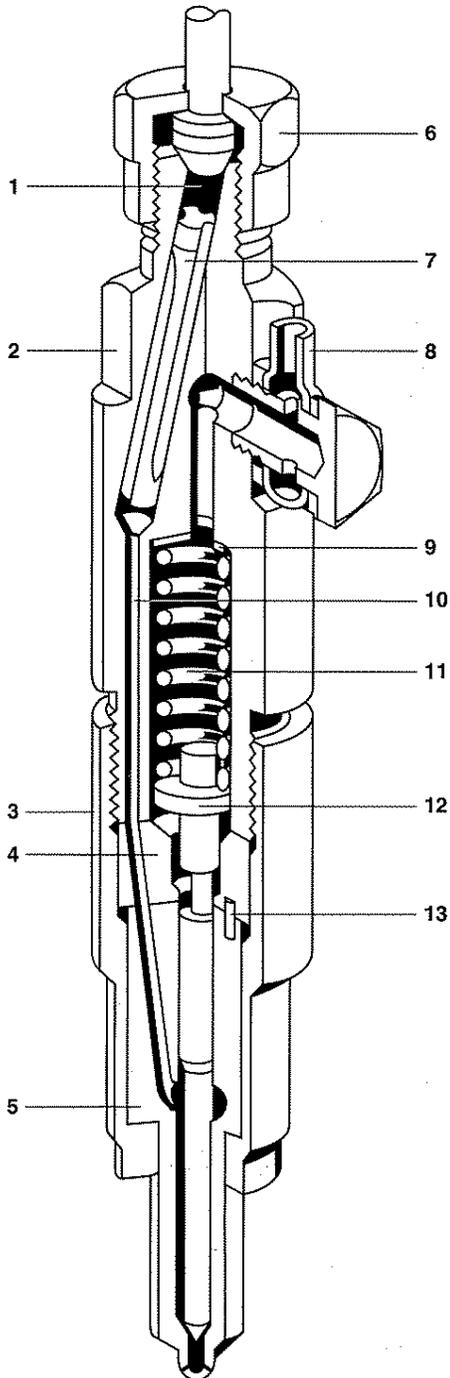
**Fig. 6: 2-spring nozzle holder KBEL...P...**
