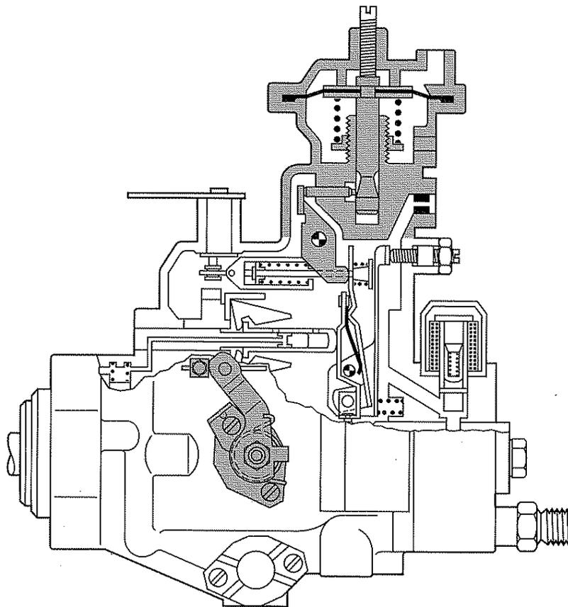
**Fig. 2: Schematic of the VE distributor pump with mechanical/hydraulic full-load torque control**
