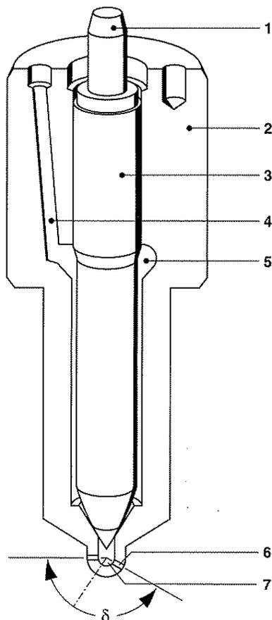
**Fig. 4: Nozzle-and-holder assembly**
