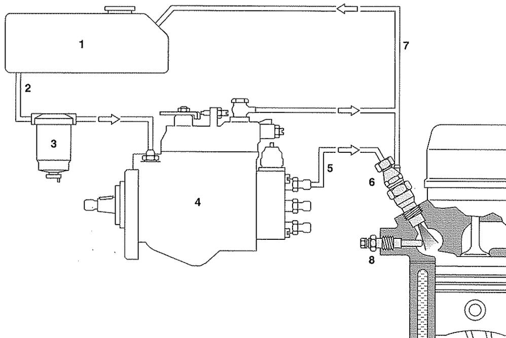
result, the vane-type supply pump in the injection pump is powerful enough to draw the fuel out of the fuel tank and to build up sufficient pressure in the interior of the injection pump.
