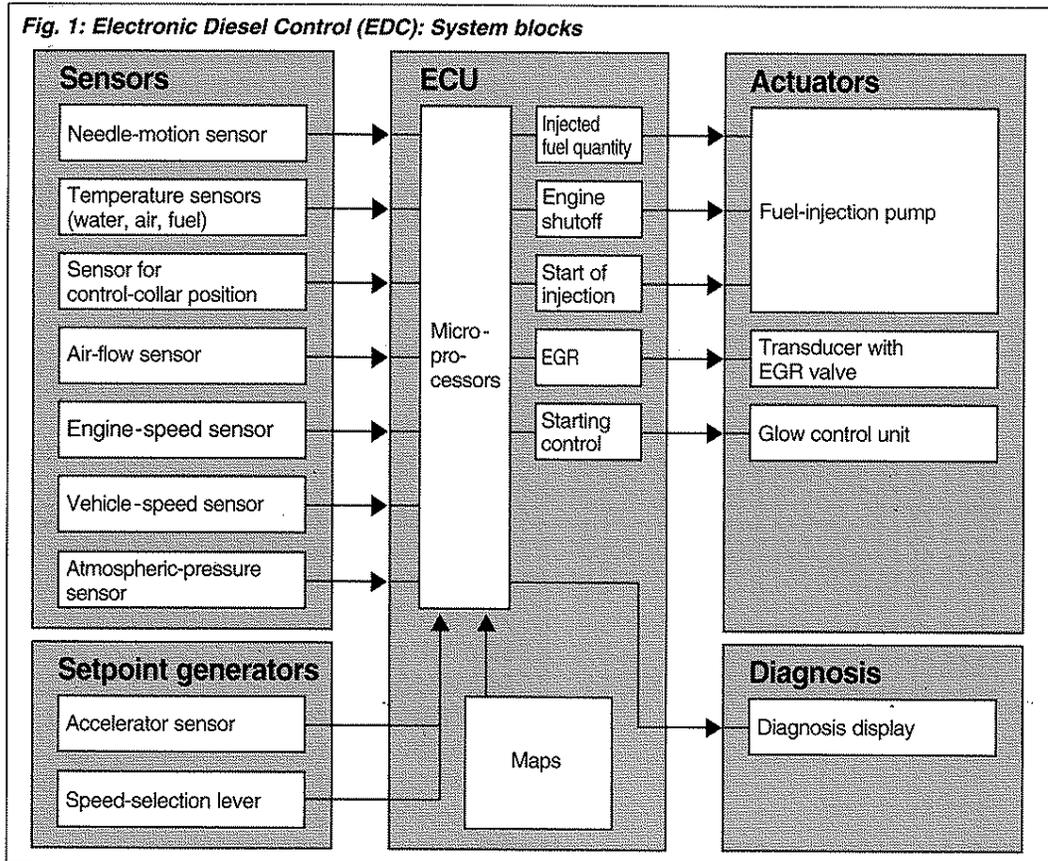
2. Electronic control unit (ECU) with microprocessors which processes the information in accordance with specific control algorithms, and outputs corresponding electrical signals.
